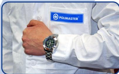
The PM1208 Wristwatch Gamma radiation Dosimeter incorporates a sensitive Geiger-Muller based gamma detector and a stylish wristwatch, combining a leading edge dosimeter technology with Swiss tradition of the watch making. An audible alarm alerts the user when a potential radiation hazard exceeds adjustable radiation threshold levels. The instrument contains non-volatile memory to keep the measured data until they are downloaded to a PC by means of built-in IR interface.
