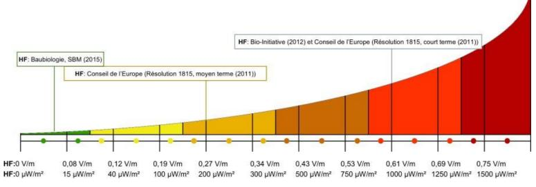
Indicative measure of radiation strength for radio frequencies (RF) in volts per metre (V/m) and microwatts per square metre (µW/m²), depending on the colour of LED switched on. The threshold values given are recommendations and standards and are taken from appropriate sources (see below).
