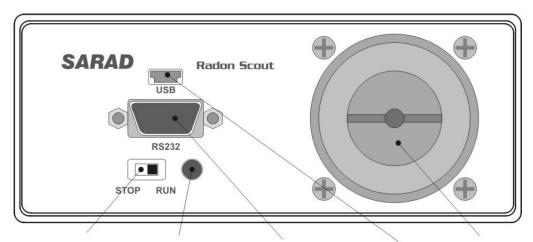
Toggle Switch Status LED Connector for Serial Cable USB port Battery Slot
